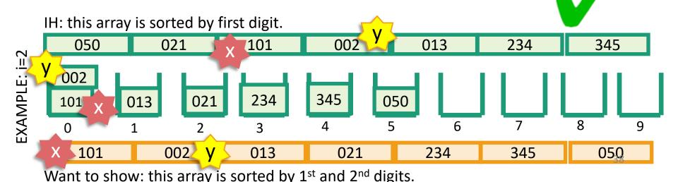
Want to show: after the i'th iteration, the array is sorted by the first i least-significant digits.
